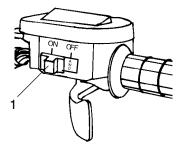
When in AWD, the front gearcase will automatically engage any time the rear wheels lose traction. When the rear wheels regain traction, the front gearcase will automatically disengage.
